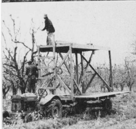
Two-stage pruning platform for pears with slip-boards on upper deck. Compressor is mounted on tractor.
