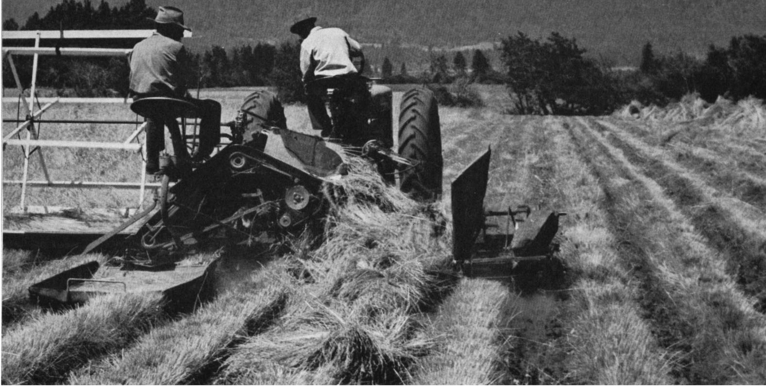
**Binders should be modified by the addition of pans under the drapers and tying platform to catch seed shattered in cutting and tying. Note short pieces of hose on reel slate which are centered on rows and help in keeping cutter bar free.**
