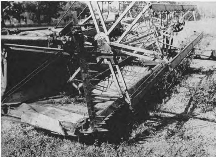
Close-up view of a windrow-swather. The vertical cutter in the foreground separates the cut material from the standing growth. The pick-up reel contributes to a cleaner job of cutting and lays the material back onto the canvas draper which conveys it to the left side of the swather.
