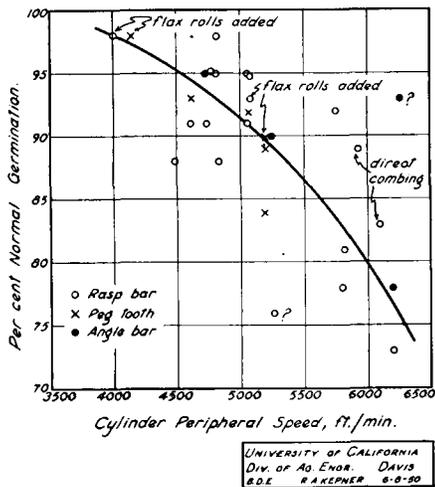
Relation of germination percentage to cylinder speed, for various types of combines. No significant differences are evident between the three types of cylinder. Seed moisture contents ranged from 5.2% to 7.5%.
