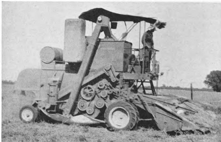
Self-propelled combine harvesting in a field with heavier-than-average windrows. The canvas sheet suspended beneath the machine catches any seed that leaks out. The ground-driven belt-type windrow pick-up was the most satisfactory type observed. The windrow here is being lifted with a minimum of disturbance.
