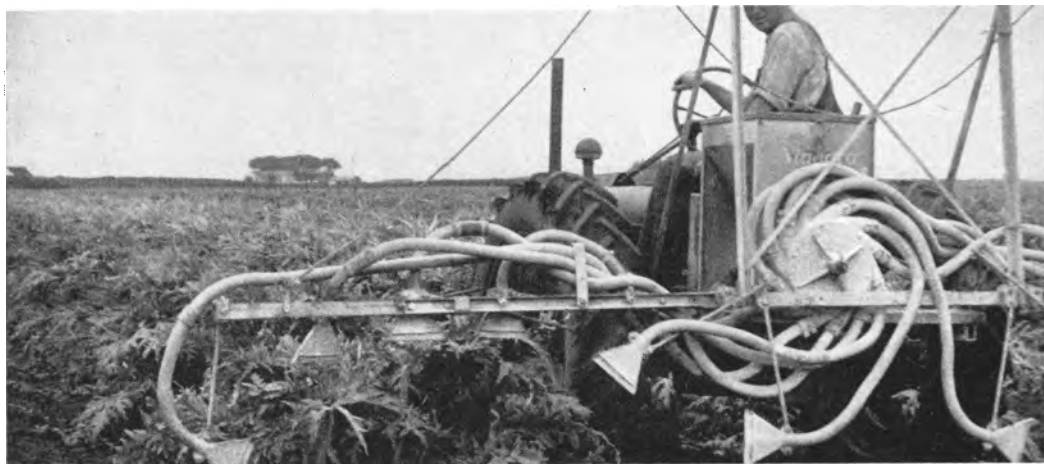
Power duster showing proper arrangement of nozzles for control of the plume moth.
