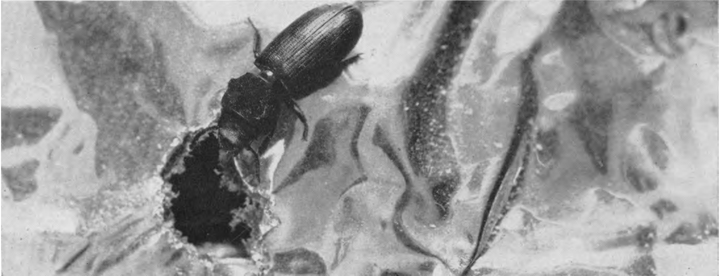
Laminated film package showing penetration by the cadelle.
