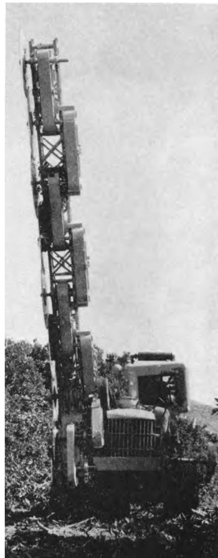
**A trailer mounted hedging machine using twelve 14" diameter saws driven by a 25 H.P. air-cooled engine. This machine is capable of hedging lemons, oranges or grapefruit on two sides of each row at the rate of ¾ to 1 acre per hour.**
