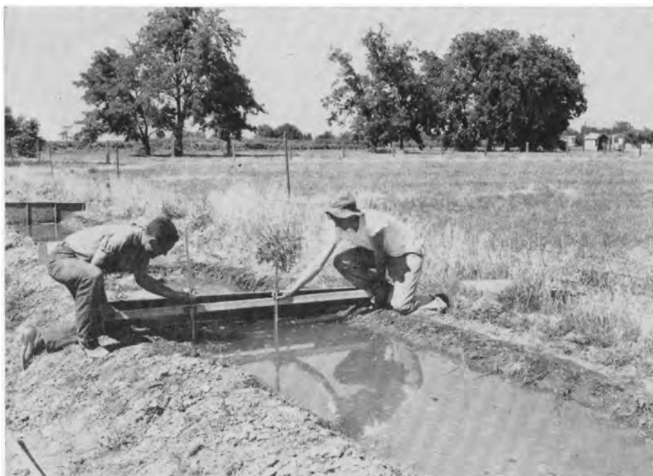
Making measurements during a seepage ponding test.
