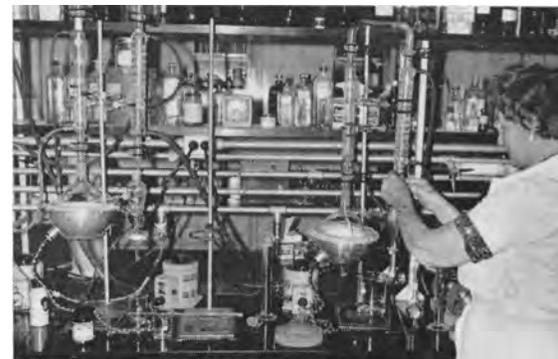
Use of this hydrolysis apparatus in the colorimetric analysis of herbicides, is one of many painstaking laboratory procedures conducted in departments at all campuses to produce scientifically exact information on the safe use of agricultural chemicals.
