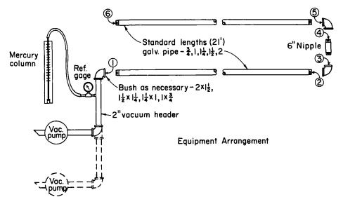
tings in terms of equivalent straight pipe can be used for milking machine considerations. The meter readings taken at elbows (points 3 and 5) were usually lower than readings taken at the end of a straight pipe or nipple. This would suggest that the nozzle effect of the airflowmeter rubber adapter, when inserted into an elbow, aggravates the turbulence loss caused by such a fitting.
