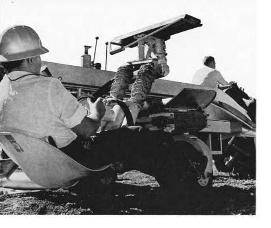
Operator of the U.C. mechanical grape harvester sits low to control the cutter bar as it removes clusters of grapes hanging below trellis. Intercom system allows operator communication with driver of tractor pulling the harvester.
