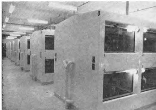
Dog cages for radionuclide treatment. Each 10-sq.-ft. cage has a shatterproof sliding glass front door and sliding partition between cages. Dogs stand on an expanded steel grate above the cage bottom and excreta are washed into a drainage line connecting directly to a disposal system. Air flows from the room through the cage and is exhausted to the outside.
