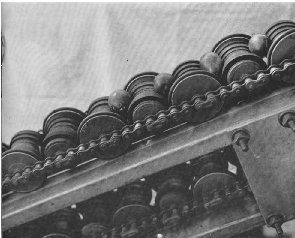
Concave rollers of specially designed conveyor positioned fresh fruit lengthwise for pitting knife in removal of pits for pitted dried prune production.
