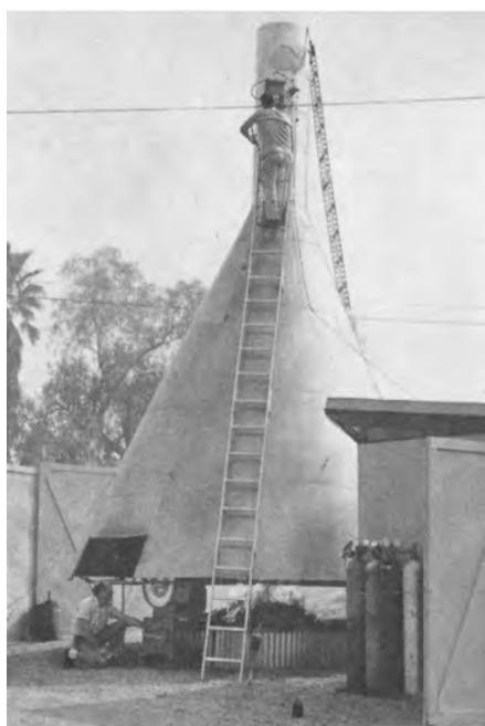
Burning tower and laboratory, to right, with technician checking scales as fuel is burned and another technician, on ladder, checking a velometer, mounted outside the upper stack, which records air flow as transmitted electronically from an anemometer mounted inside.
