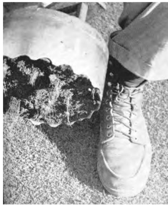
After removal of  $1\frac{1}{4}$  to  $1\frac{1}{2}$  inches of thatch and soil, the penetration rate was  $\frac{1}{4}$ -inch per hour. When 4 to 6 inches of the stratified, compacted material was removed, the parent soil was found to have a rate of infiltration of approximately 2 inches per hour.
