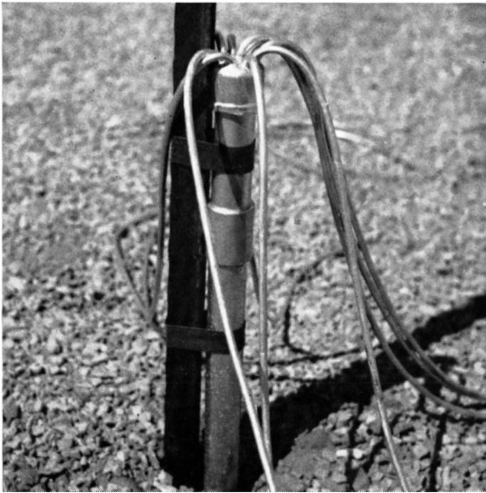
Plastic cap on each riser is drilled to take nine 48-inch plastic tubes.
