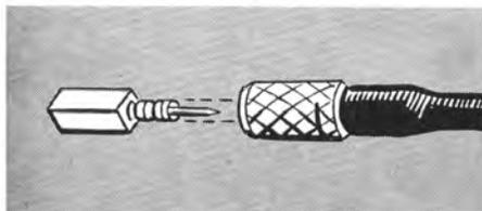
Drawing above shows nozzle connected to flexible tubing with adjustable pin to left. Cross section, below, shows flexible tubing tap as connected to main line.
