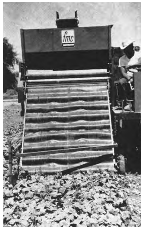
Front view, above, of FMC once-over harvester for pickling cucumbers showing pick-up mechanism. Below left, close-up of cutting and pick-up mechanism of FMC harvester; right, delivery belt carrying cucumbers from harvester to bins.
