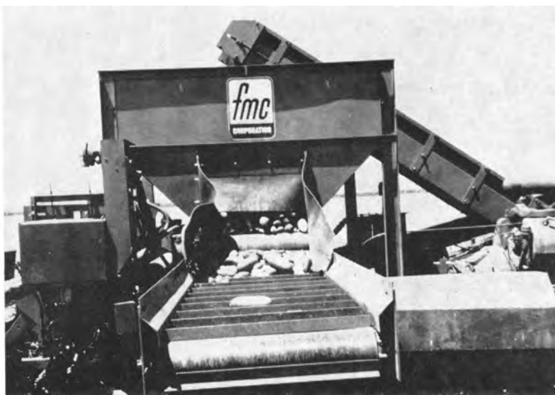
Front view, above, of FMC once-over harvester for pickling cucumbers showing pick-up mechanism. Below left, close-up of cutting and pick-up mechanism of FMC harvester; right, delivery belt carrying cucumbers from harvester to bins.
