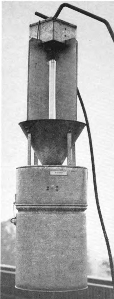
Blacklight insect trap with omnidirectional-positioned 6-watt lamp.
