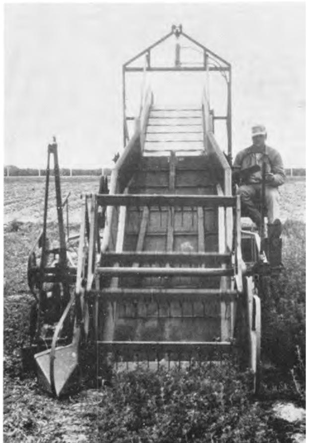
U.C.-built alfalfa plot harvester designed for harvesting and weighing small plots.
