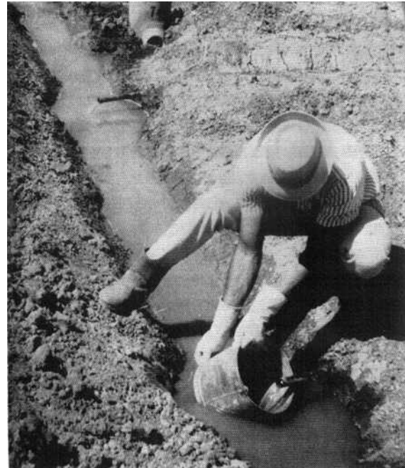
Inflow and outflow rates were measured with a known volume of irrigation water and a stop watch.
