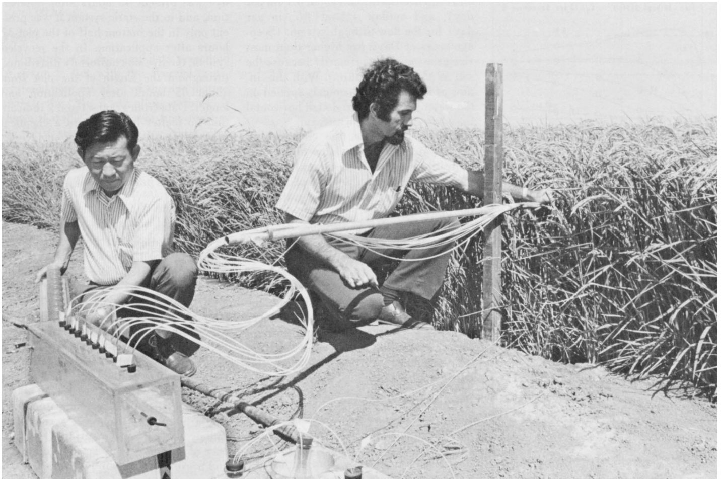
Flood water sampling equipment for chemical residue tests with dye tracers in rice.
