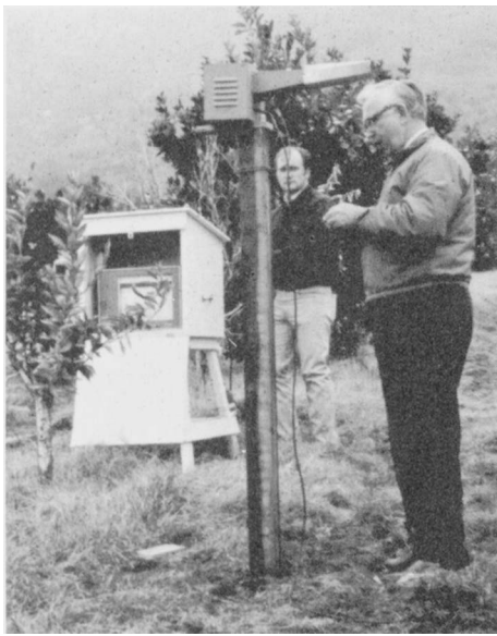
One of two temperature and radiation monitoring stations used in these frost protection tests at the Topa Topa Ranch, Ojai.
