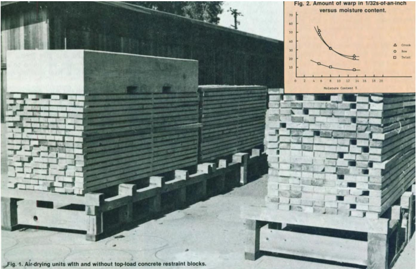
Fig. 1. Air-drying units with and without top-load concrete restraint blocks.
