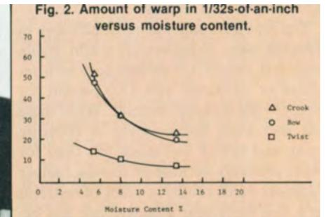
Fig. 2. Amount of warp in 1/32s-of-an-inch versus moisture content.
