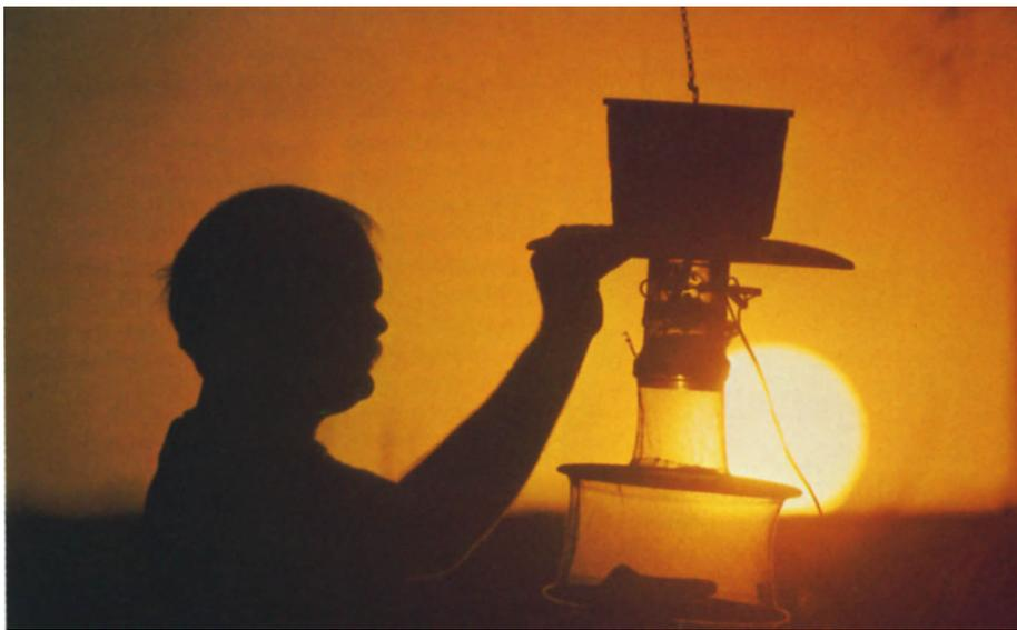
Carbon-dioxide light trap is used, along with other baited traps, to collect mosquitoes in studies of virus transmission.
