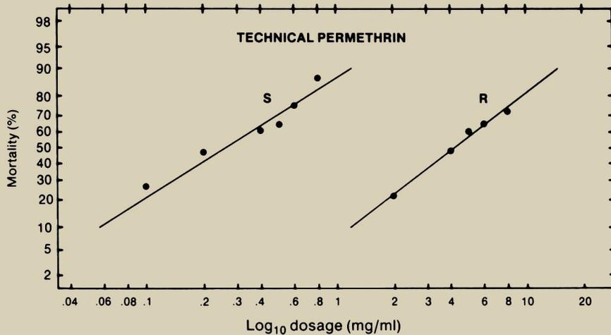
**Dose-response lines of susceptible (S) and suspected resistant (R) strains show development of resistance in R strain. (Each data point is a mean from 80 adult female flies less than 3 days old.) LD<sub>50</sub> values can be obtained by reading across from the 50% mortality value to the S and R lines, and then down to the dosage value.**
