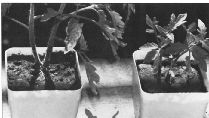
Plant growth in stabilized soil (left) compared with nonstabilized soil. Both had been subjected to heavy watering.
