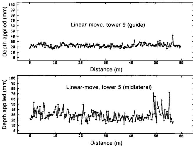
Fig. 1. Uniformity of the linear-move machine varied more near midlateral tower (lower graph) than near guide tower (upper).
