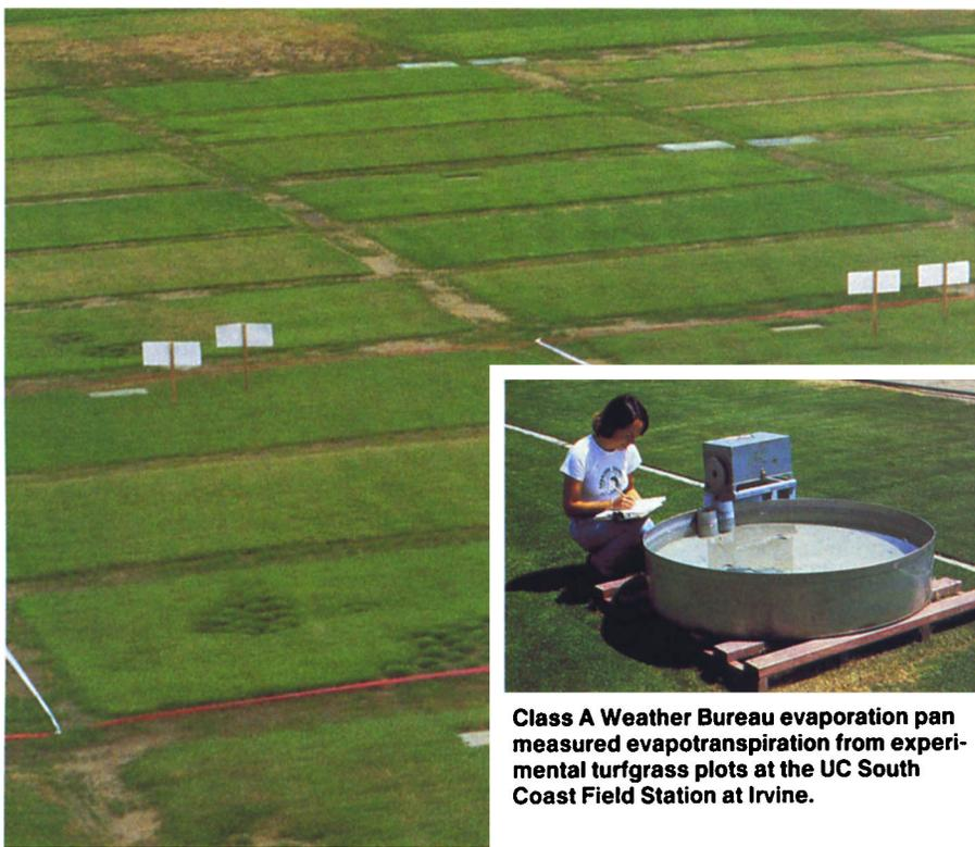
**Class A Weather Bureau evaporation pan measured evapotranspiration from experimental turfgrass plots at the UC South Coast Field Station at Irvine.**
