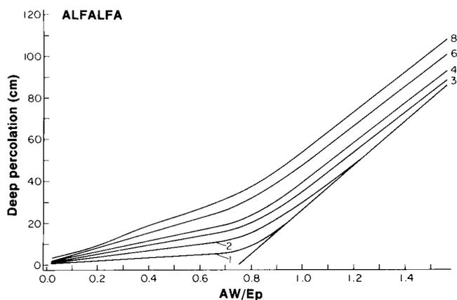
**Fig. 2. Computed values of deep percolation when alfalfa irrigated with various quantities of applied water at a given dSm. Increasing application of brackish water increases the volume of drainage water.**
