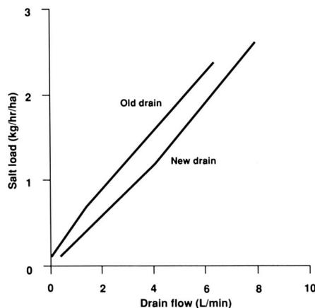
Fig. 2. Same drains show direct relationships between salt load and flow rate.
