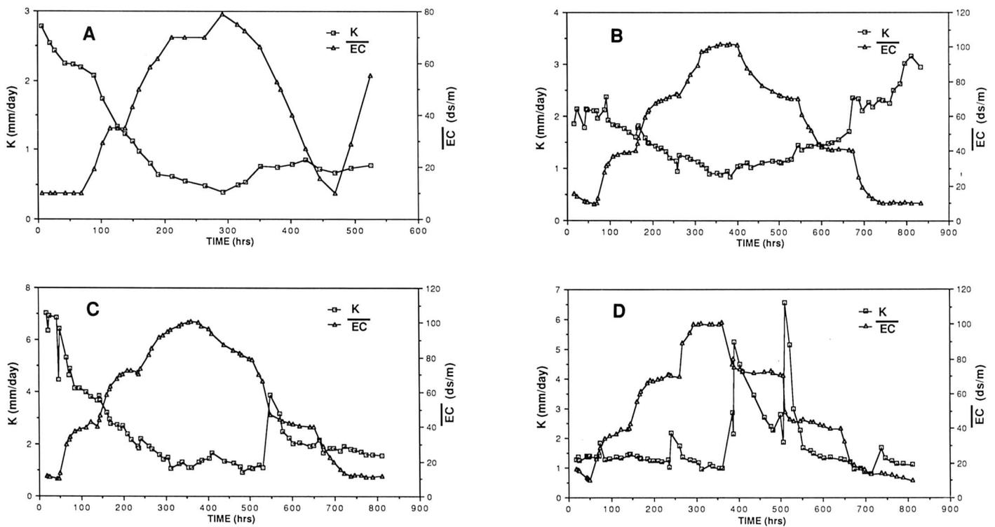
Fig. 1. When percolating drain water was nonsterile (A and B), permeability,  $K$ , decreased as mean salinity,  $\overline{EC}$ , increased. Permeability declined irreversibly as time of ponding increased (A) but rose again in relation to a decrease in salinity (B). When drain water was nearly sterile (C and D), permeability tended to decrease with time (C) and showed only temporary, erratic changes at higher salinity levels.
