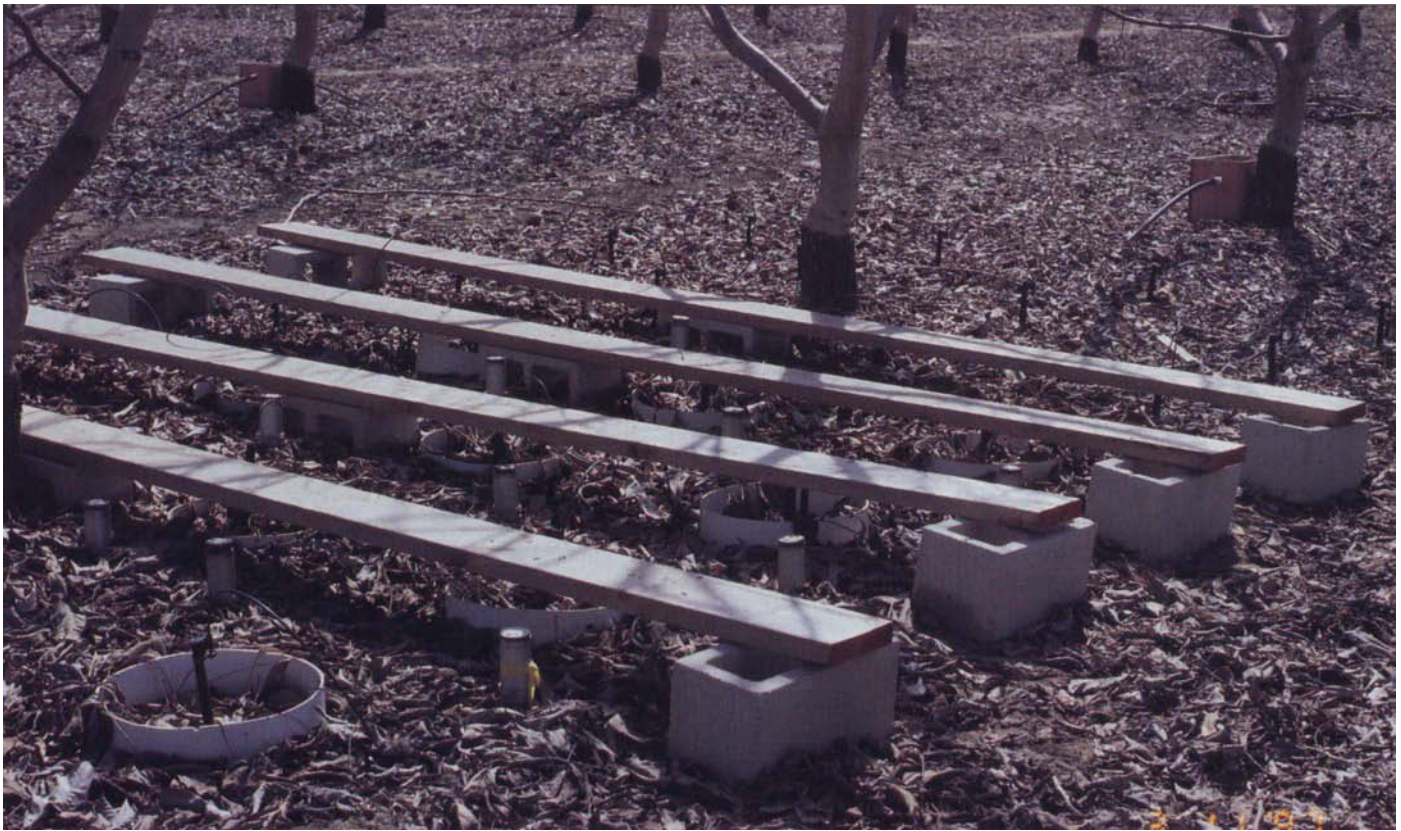
Neutron probe access tubes in hedgerows were used to assess changes in soil water content. Drip emitters in the monitored root zone quadrant were located on stakes and surrounded by rings to limit overland flow. Boards facilitated access to tubes for data collection.
