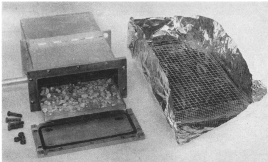
Fig. 14. The vacuum tank unit, showing the lower tray containing calcium hydride lumps and the upper tray containing plants ready to be freeze-killed. The aluminum foil wrapping around the plant tray is pulled down at the front to show construction of the tray.
