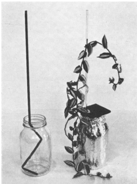
Fig. 6. The quart Mason jar on the left shows a plant support made of glass tubing; on the right, the plant support holds a Tradescantia plant in position.
