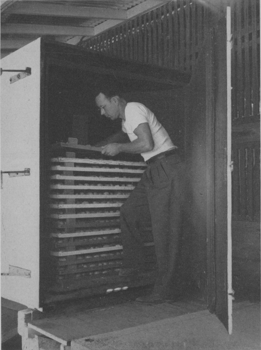
Fig. 7. Interior of fumigation box. The trayed potatoes are exposed to 55 cc methyl bromide for 2 hours at 80° F.
