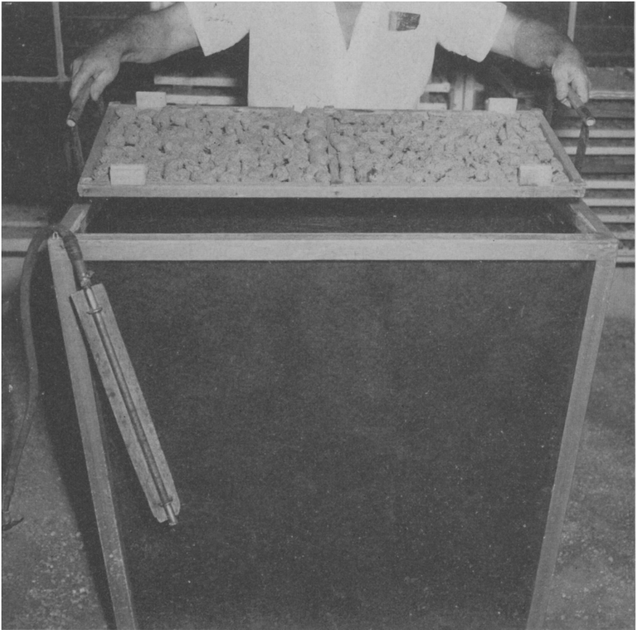
Fig. 10. Metal tray holders being used to set tray of mother scale inside top of scale transfer hopper. Note air brush consisting of a perforated brass tube fastened to a board for ease in handling.
