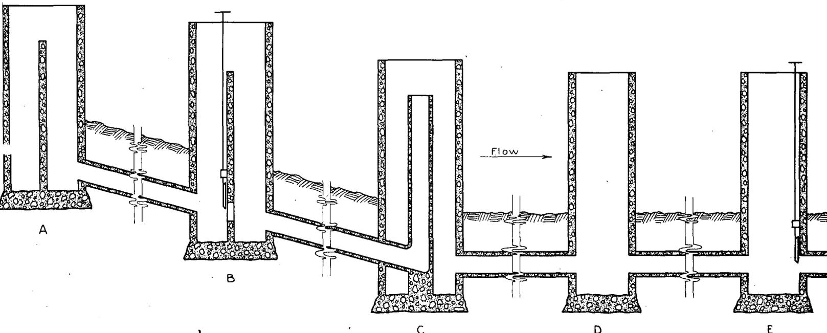
Portions of an open concrete pipe irrigation distribution system. Deliveries are at the upstream end of each stand. A is an overflow stand; B is an overflow stand with a gate in the baffle wall; C is an overflow stand consisting of a riser pipe within the larger stand; D is a simple stand; E is a simple stand with a gate over the outlet.
