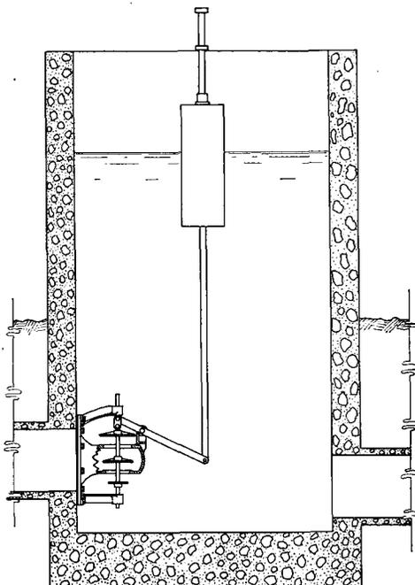
A float valve stand as used on semiclosed systems.
