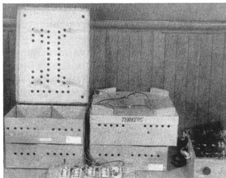
Equipment used in determining the effect of temperature inside chick and poult boxes. Wires lead to thermocouples inside boxes.
