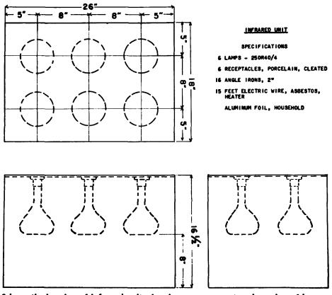
Schematic drawing of infrared unit, showing arrangement and spacing of lamps. Wiring—not shown—is arranged in parallel.
