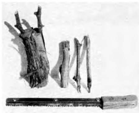
Hand saw for notching stock in field and scions having a single tongue.
