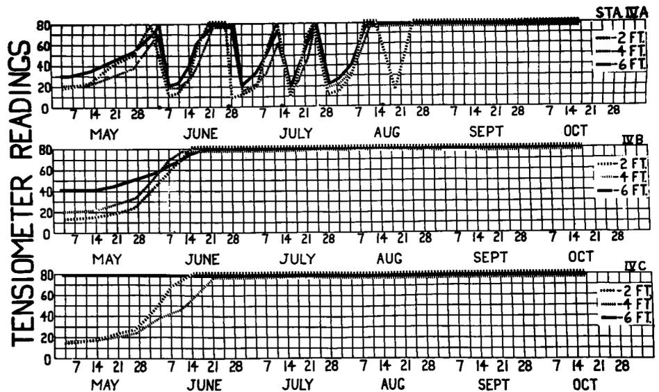
Tensiometer readings, showing the inadequate irrigation of grapes by use of a single furrow every other vine row.
