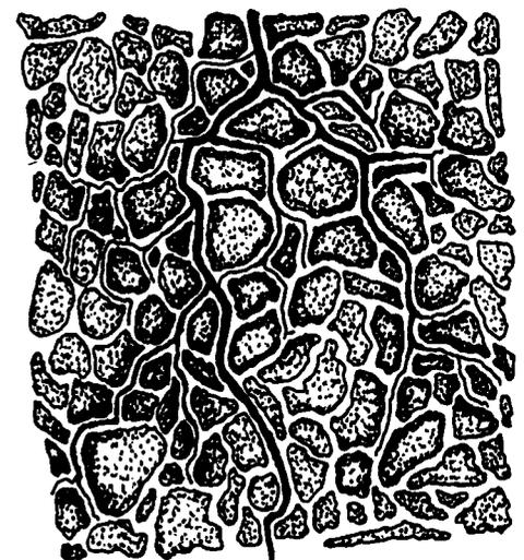
Schematic diagram illustrating the manner in which soil additives spread through small and large pores.
