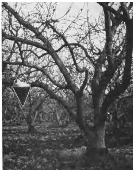
Black light trap hanging from walnut tree in a northern California orchard. Black light tube is mounted horizontally across top rim. Galvanized tin funnel tapers down into a quart jar for insect collection.
