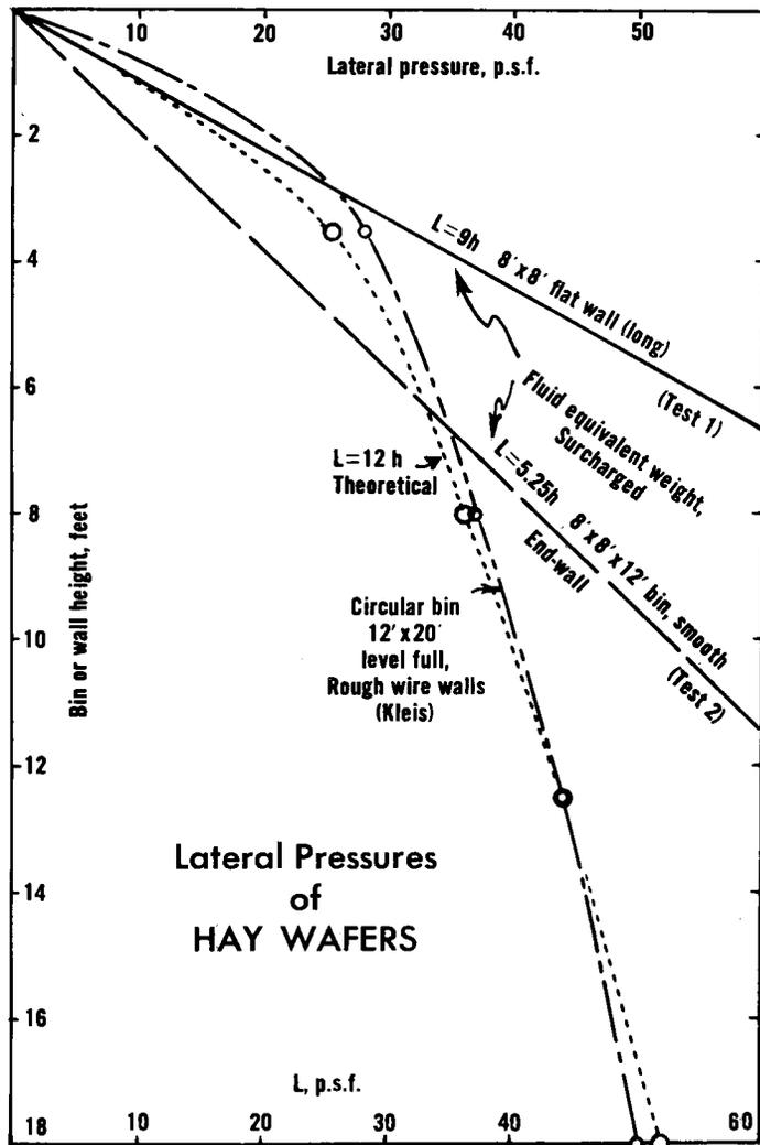
In each test, wafers were piled against the wall with a drag-type elevator—delivering the wafers at a point 4 to 6 ft from the wall and high enough to form a normal cone with a 45 degree angle of repose at maximum wafer depth. This provided surcharge storage conditions on the pressure walls. Wafers contacted the walls along a curved or conic section, and average height was carefully estimated.
