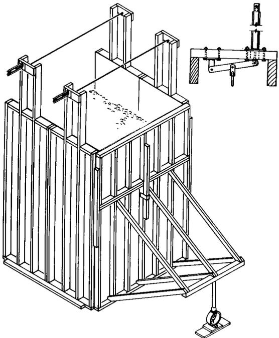
Drawing of pressure walls used in second test. Tension scales are shown at left top. Multiplier is shown in detail. Pile of wafers formed the fourth side of bin.
