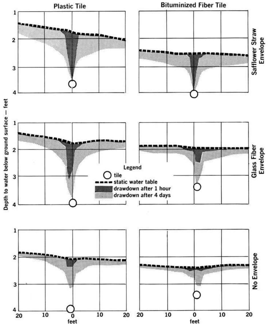
Water table profiles perpendicular to field drain tile lines, showing static water table and drawdown after one hour and again after four days. Tile indication on graphs is diagrammatical (not to scale) and only open tiles are shown.
