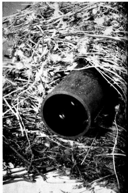
Four-inch bituminized fiber tile with 5/8-inch perforations, in safflower straw envelope.
