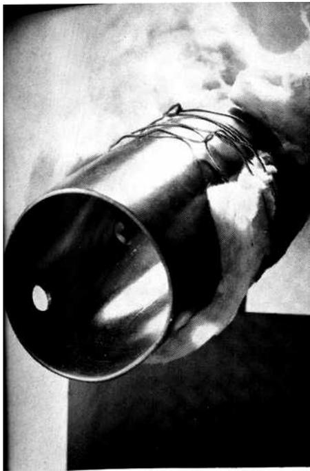
Four-inch plastic tile with  $\frac{5}{8}$ -inch perforations, wrapped with glass fiber envelope.
