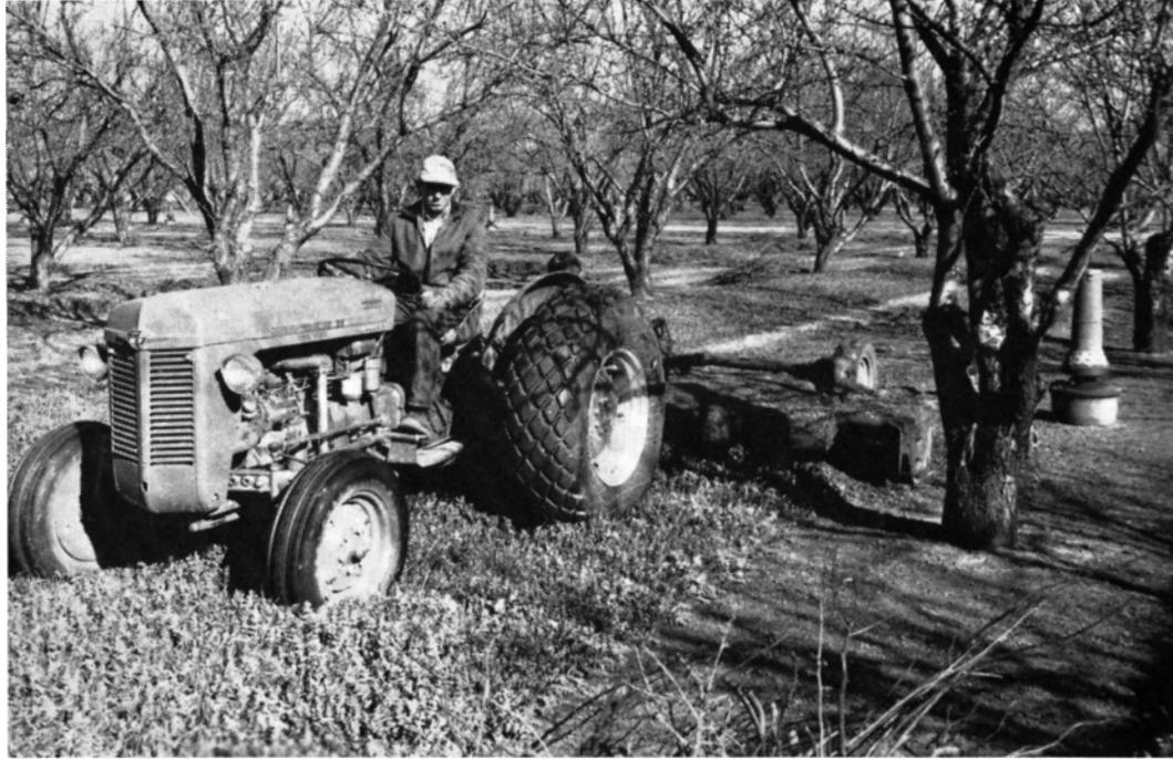
Rotary chopper seen above is typical of type used in orchard mowing for nontillage system.
