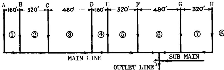
Stations (1), (2), and (3) in line layout sketch above were recorder wells. Stations (4) through (8) were observation wells only. Line details are specified in table below.
