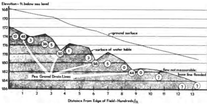
Graph 3. Profile of John Jones orchard, Mecca, Oct. 28, 1966, during an irrigation (same methods and notation as in graph 1). New pea gravel lines were carrying most of the water, had no water over them, and had lowered the general water table. (Water flow calculations were made by G. J. Hoffman, U.S. Salinity Laboratory, Riverside.)
