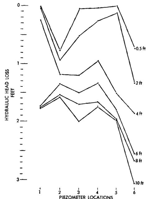
Hydraulic head loss in the gravel of the stream channel where no surface sediments were present. The numbers at the right denote the depths of the piezometers.
