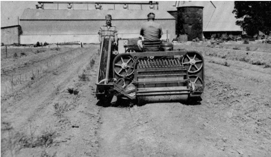
U.C. nonselective asparagus harvester. A hand-cut row is at the immediate right of the harvester and a selective machine row is adjacent on the left, both of which were disked 26 days earlier. The second row to the left is a nonselective row just before harvesting.
