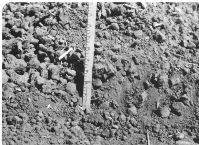
Regular bed showing surface and profile to 3-inch depth. Aggregate size distribution in top 2 inches, over 12 mm (½ inch) 35%, 0.5 to 12mm 43%, below 0.5mm 22%. Note pockets of small and large particles. Thousands of acres of crops are planted to beds such as this each year.
