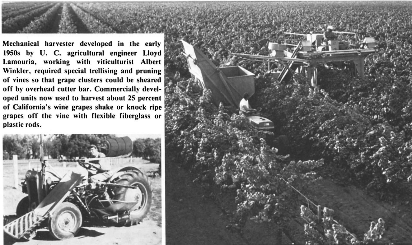
Mechanical harvester developed in the early 1950s by U. C. agricultural engineer Lloyd Lamouria, working with viticulturist Albert Winkler, required special trellising and pruning of vines so that grape clusters could be sheared off by overhead cutter bar. Commercially developed units now used to harvest about 25 percent of California's wine grapes shake or knock ripe grapes off the vine with flexible fiberglass or plastic rods.
