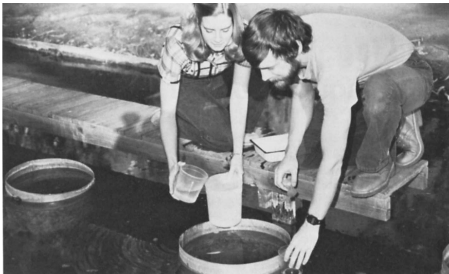
University scientists investigate the effectiveness of an oviposition repellent in preventing gravid mosquitoes from laying eggs. Sheet-metal cylinders dispense the repellent in experimental ponds.
